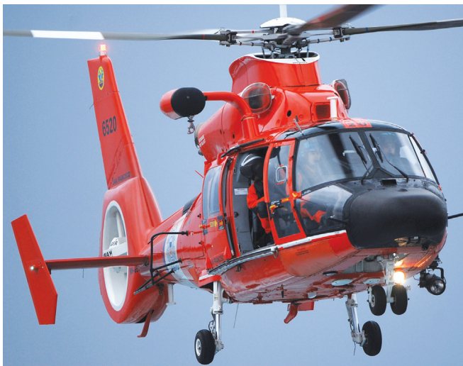
The HH-65 Dolphin, which entered service in the early 1980s, has been modernized into its current designation of MH-65, with the addition of replacement engines, glass cockpit and other enhancements.
