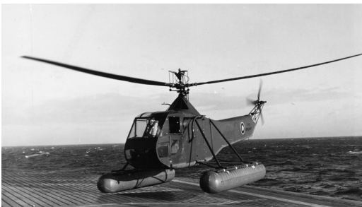
Coast Guard Helicopter Pilot No. 2, Stewart Graham, lands a YR-4 (HNS-1) helo on the British freighter SS Daghestan in 1944 while en route to Liverpool from New York. Stewart was assigned as the project helo pilot aboard this vessel to evaluate the feasibility of utilizing helos aboard merchant ships for anti-submarine patrols around the convoy.
