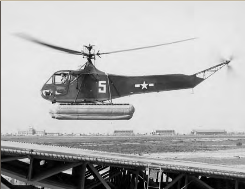
A Coast Guard HNS-1 Hoverfly pictured during tests on a rocking platform simulating a rolling ship deck that was constructed at Coast Guard Air Station (CGAS) Brooklyn (Floyd Bennett Field), New York, 19 May 1944. (NNAM)
